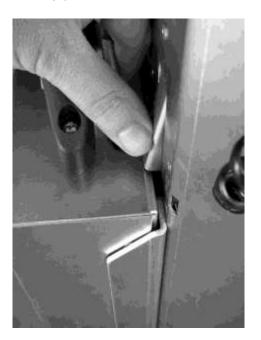
4. While pressing the battery-pack lock button, pull the battery-pack up and out.
