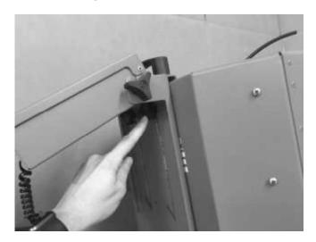
2. Pull up on the handle until it stops and then lower the handle at an angle to lock in place. Tighten the triangle head screws.
